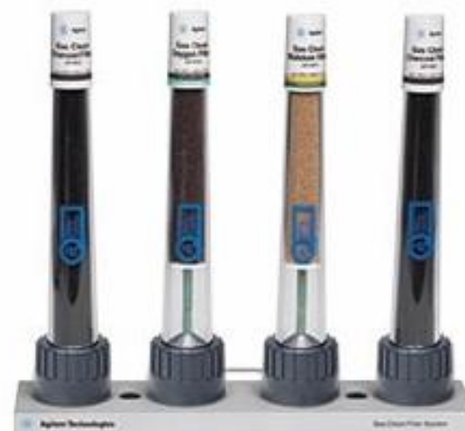
Gas Clean purification system
