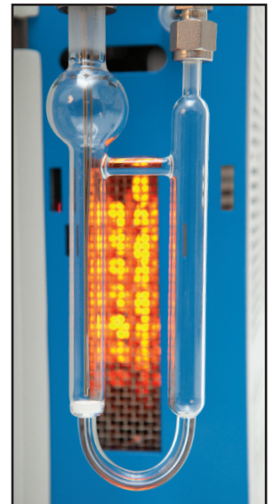
Figure 4. Sparge Tube Carry-Over Reduction System
